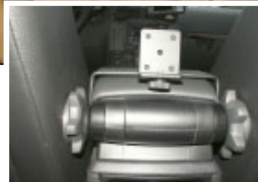
A between seats monitor mount for monitors with thumb screw attachment, Tablet DVD in place.
