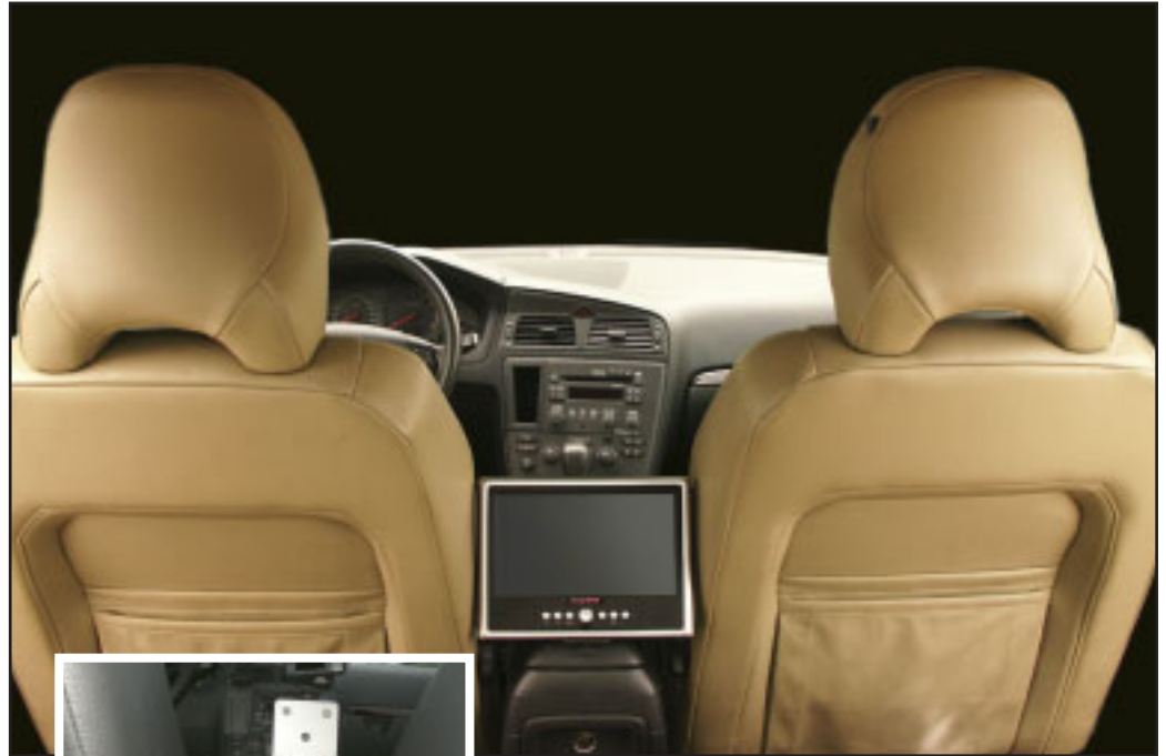
A between seats monitor mount for monitors with thumb screw attachment, Tablet DVD in place.
